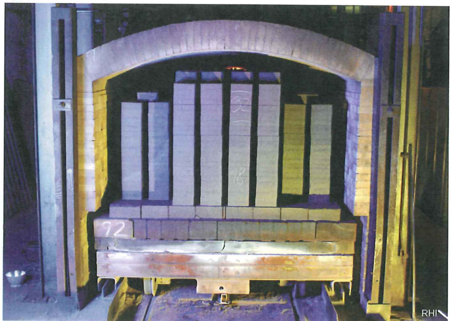
Refractory bricks entering a tunnel kiln
